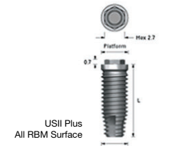
Fig. 1. USII Plus implant (Diameter:4.0mm, Length:13mm).
