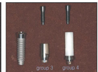
Fig. 2. Internal octagonal implants, abutments and abutment screws (group 3: Titanium abutment, group 4: UCLA-type abutment).
