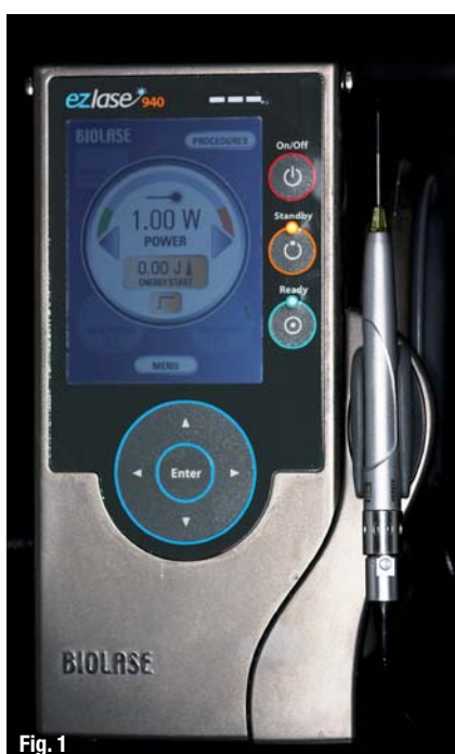
Fig. 1_ The 940 nm diode laser that was used for this study: Ezlase 940, Biolase®.
