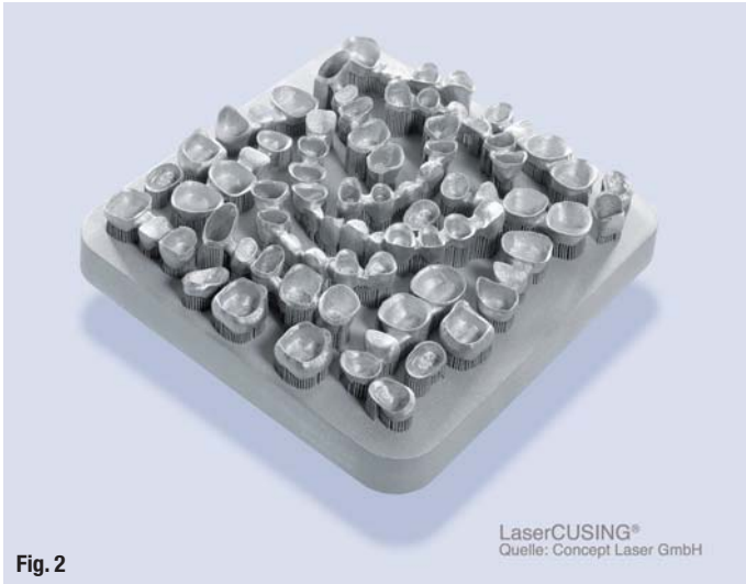
Fig. 2 Crowns and bridges manufactured using laser melting technology.
