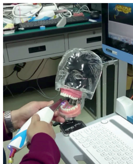
Screenshot (YouTube/solberg hu) of the newly developed blue laser line intraoral scanning device (MIRDC Taiwan).
