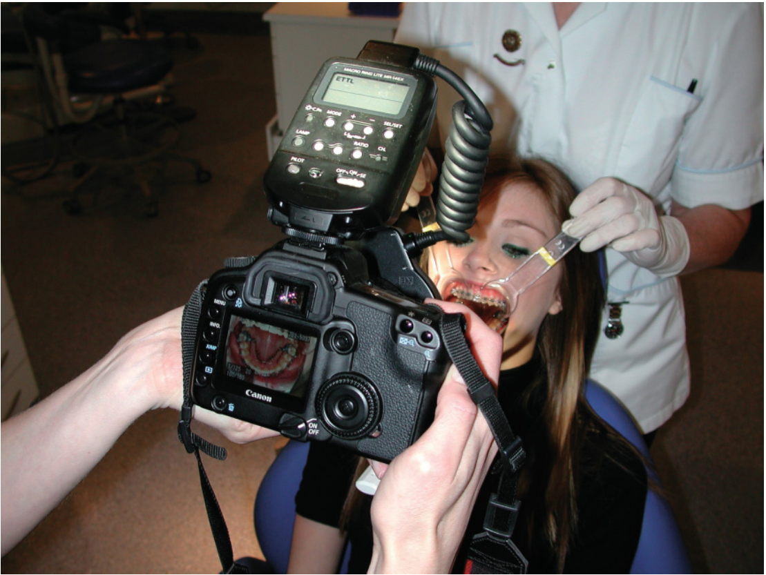
Figure 8.1 LCD screen in 'live view' mode to allow shot to be composed easily.
