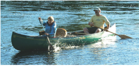
Figure 29.1 Newton's third law of motion in action. The canoe is being propelled forward by the backward force of the paddling.
