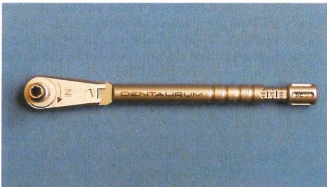
FIGURE 10-47 The driver for some screws is made so that it will not deliver more than a controlled amount of torque, which decreases the chance of fracturing a screw or overstressing the bone.
