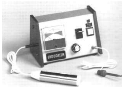
FIG. 14-40 Endocator canal measuring device (Hygenic). Insulated probe not shown.
