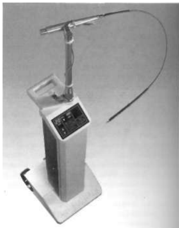
FIG. 14-46 Carbon dioxide laser unit (Luxar, Bothell, Wash) with flexible waveguide for intraoral use.
