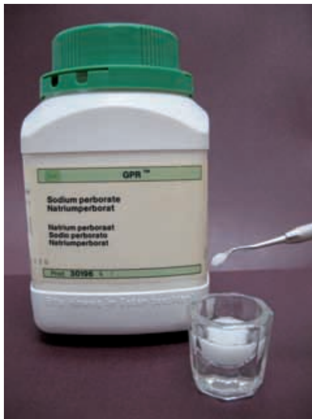
Figure 6 Sodium perborate powder and water are mixed to a thick consistency of wet sand.
