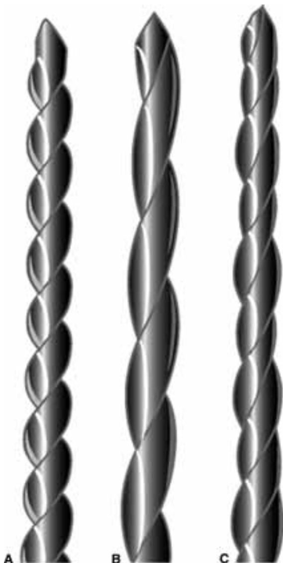
Figure 3 ISO Group I, K-style endodontic instruments. A , K-style file. B , K-style reamer. C , K-flex file.
